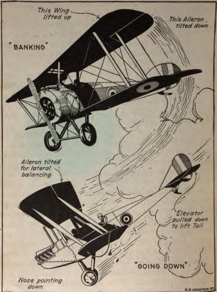
Fig. 97. Illustrations Showing How Control Elements are Moved to Regulate Airplane Flight.
